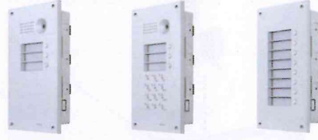
9135511E Vandal resistant mask and box for masonry fitting Mask: 138,5 x 241 mm Hole: 110 x 220 x 50 mm 9135511KE Vandal resistant mask with keypad and box for masonry fitting Mask: 138,5 x 241 mm Hole: 110 x 220 x 50 mm 9135515E Vandal resistant mask and box for masonry fitting Mask: 138,5 x 241 mm Hole: 110 x 220 x 50 mm
