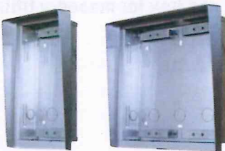
9135361E Roof & box for masonry fitting - 1 module 129 x 240 x 41 mm Hole: 110 x 220 x 50 mm 9135362E Roof & box for masonry fitting - 2 modules 229 x 240 x 41 mm Hole: 210 x 220 x 50 mm
